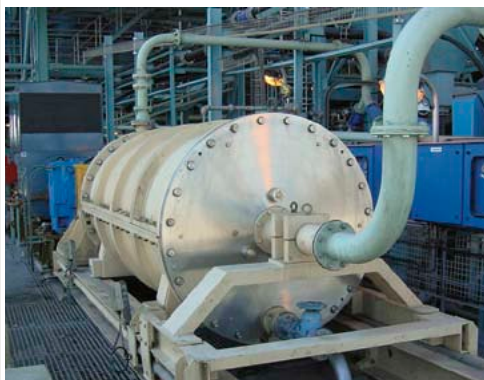
The M3000 IsaMill Installed at Lonmin, South Africa
